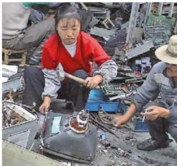
Photo: breaking cathode ray tubes (CRTs) will release cadmium containing internal phosphorous coating, which will be inhaled by the workers (source: © 2006, Basel Action Network BAN)
