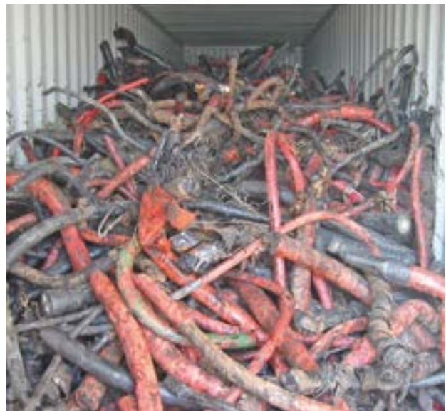
Photo: Oil coated ground cable, declared as copper waste (source: © Huib van Westen, Human Environment and Transport Inspectorate, the Netherlands)
