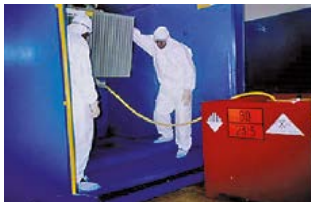
Photo: sampling of PCB containing transformers (source unknown)
