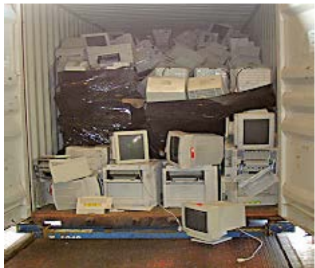
Photo: badly stowed and packaged monitors (source: © Dutch ILT)
